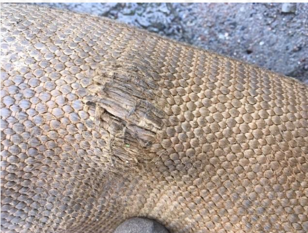
Cover is damaged by cuts
