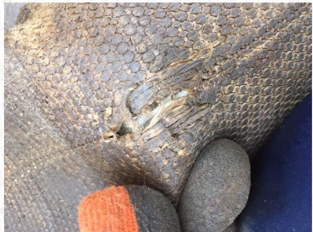
Cover is damaged by open seam
