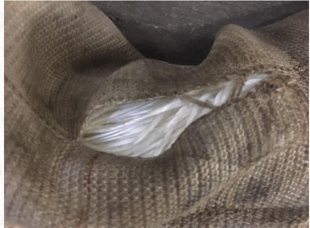
Cover is damaged by open seam
