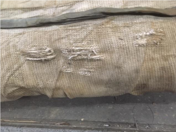
Cover is damaged by cuts
